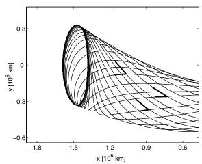
Fig. 5 Velocity wedges and a manifold of an HLO; orbits with velocity interior to the wedge are transit orbits, orbits with velocity on the boundary of the wedge are asymptotic, and orbits with velocity outside the wedge are nontransit.
