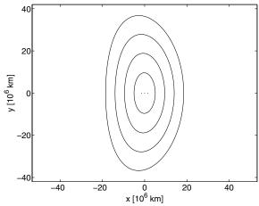
Fig. 1 Representative distant retrograde orbits; the three dots in the middle of the plot are  $L_1$ , the Earth, and  $L_2$  (from left to right).
