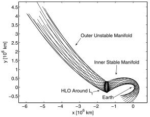
Fig. 4 Stable and unstable manifolds around  $L_1$ ; the HLO has a semiminor axis of  $90 \times 10^3$  km.
