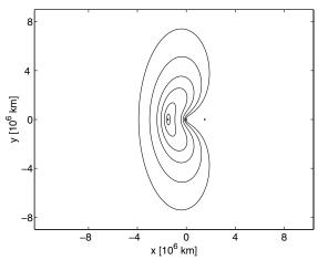
Fig. 3 Examples of EROs and HLOs around  $L_1$ ; dots in the figures represent  $L_1$ , the Earth, and  $L_2$  (from left to right); small, nearly elliptical, orbits are HLOs; larger orbits are the so-called EROs.
