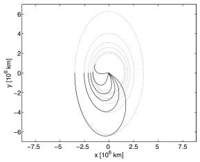
Fig. 9 Optimal transfer trajectories to selected small DROs.
