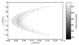
Fig. 2 Phase-space structure around a  $16 \times 10^6$  km DRO illustrated using a Poincaré section at x=0 and dx/dt>0; every trajectory on this section has the same Jacobi constant, the fixed point represents the DRO, the closed curves around it indicate the presence of invariant tori, and the gray scale indicates return times in days.
