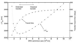
Fig. 10 Required  $\Delta V$  and travel time as a function of the target DRO semiminor axis. Combined classical transfer (right side) and extended transfer (left side).
