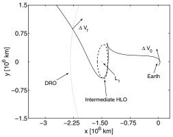
Fig. 11 Transfer from LEO to DRO using the transit orbit approach.
