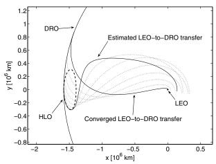
Fig. 8 Initial manifold trajectory guess converges onto an optimal transfer trajectory.
