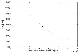
Fig. 12 Required  $\Delta V_f$  for the transfer to a DRO with semiminor axis  $4 \times 10^6$  km for different intermediate HLOs or EROs.
